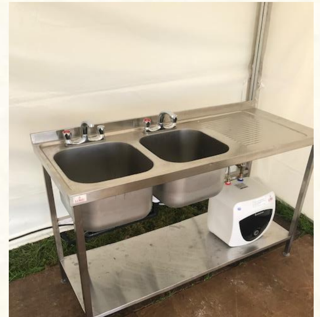
Sinks for washing up, with hot water
